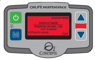
The system will begin by testing the High Priority Alarm. The High Priority Alarm consists of a 10-beep sequence separated by 2.5 seconds of silence, and the LCD screen flashes red.
