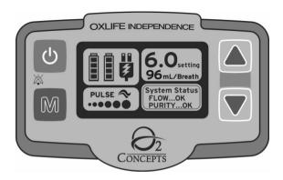
The device may take up to three (3) minutes to warm-up and reach desired performance. System Status will show Flow and Purity are OK when warm-up is complete.
