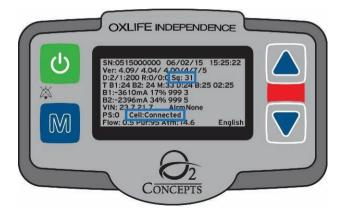
The cell signal strength is listed in the third row on a scale of 0 through 31 (ex. Sg:31). The cell status is listed in the eighth row (ex. Cell: Connected).
