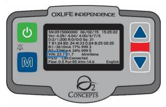
The voltage in is the voltage that the unit is receiving from an external power source, such as the AC power supply or DC power supply (ex. VIN: 23.7 where 23.7 is in volts).
